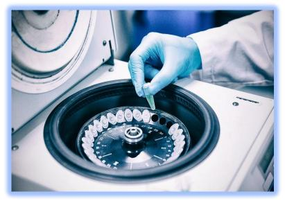
2) Centrifugation is the process of separating heterogeneous systems in the field of centrifugal forces using solid or liquid-permeable partitions. Centrifugation processes are carried out in centrifuges. During ultra-high-speed rotation, a centrifugal force occurs in the system, which contributes to the separation of the processed substance by density. The method of centrifugation is used in science
